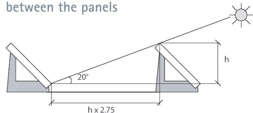
Diagram to find out the azimuth angle, in relation to the day light and shadow casting objects.
