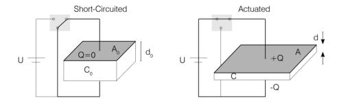
If the supportive frame is flexible, due to the initial prestretching of the acrylic film, the frame bends. After application of voltage, the material expands, and the component flattens out.
