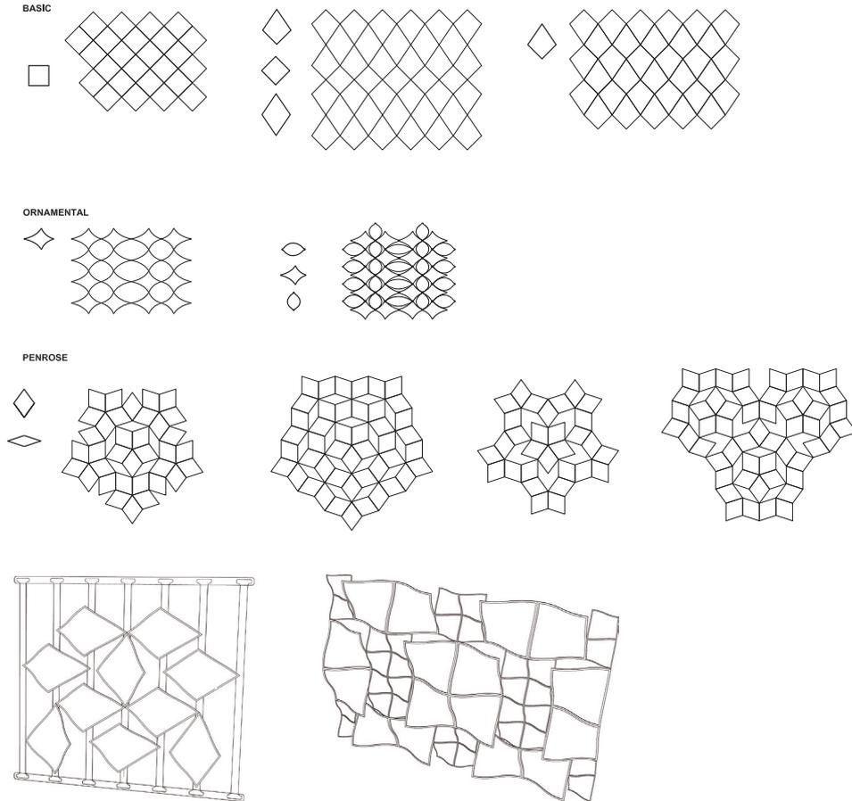
Initial investigations focused on static supporting structures for the components. After a number of experiments on static structures the interest moved towards developing dynamic structural arrangements.
